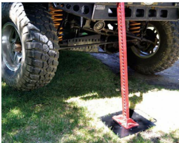
FLAT FOOT. The strength of a high-lift jack means you can lift your vehicle high into the air, but make sure to put it on a base plate on softer terrain.
